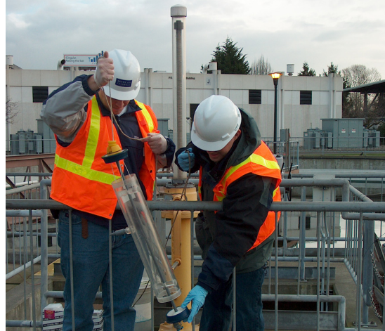
Figure 4 // BC process expert Rick Kelly performing full-scale stress testing on a clarifier.
