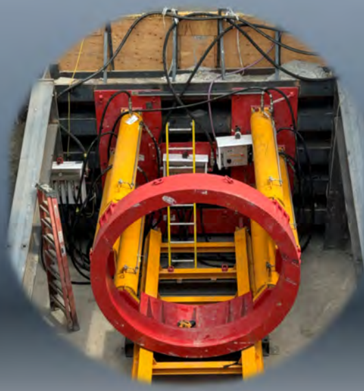
Close-up view of the Hydraulic Microtunnel Boring Machine (MTBM) Jack.
