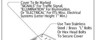
Lift Eve Junction Box Cover With Recessed Lifting Eye Or Max. 3/8" Lift Hole —
